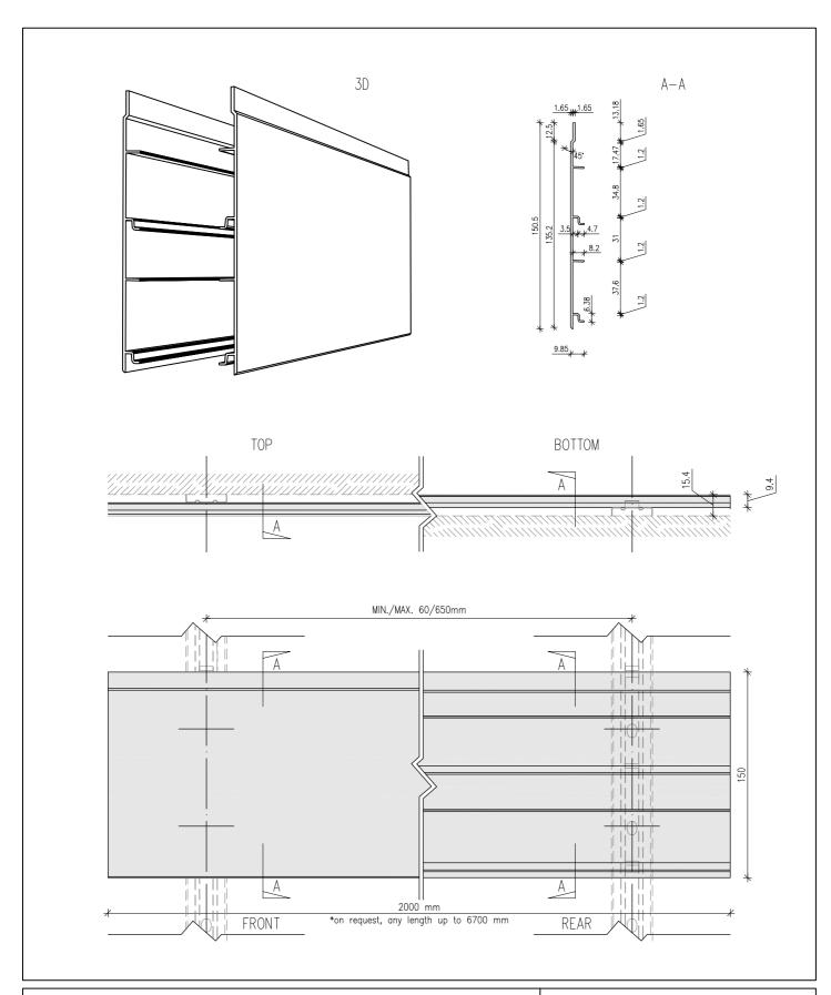
INFO: Highest fire resistance class A1. Manufacturer's warranty 20 years. Total cladding thickness only 17 mm.
